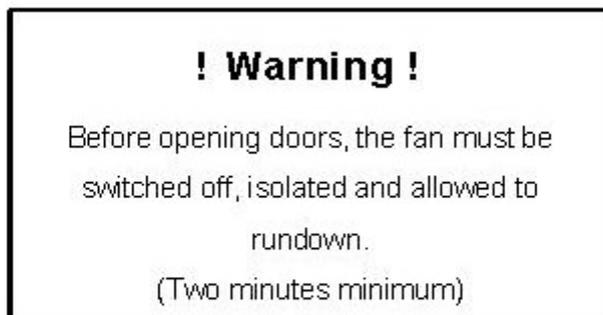
**Figure 11 — Example of text included in the warning sign for an air handling unit**
