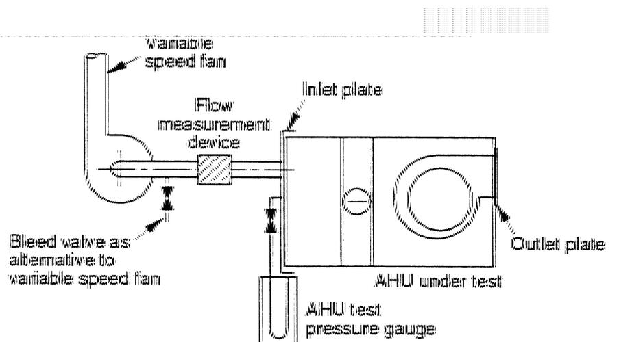
Figure 4 — Apparatus for testing the casing air leakage (negative pressure test). Typical example
